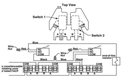
NOTE: Common and B connections will close when valve moves 1/5 of its total travel distance.
