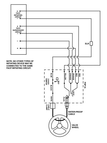
Figure 5. Multiple devices Class A:
