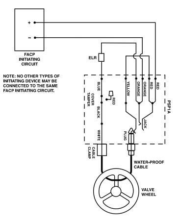
Figure 2. Single device Class B:
