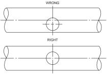
REMOVE BURRS FROM EDGE OF HOLE. CLEAN OUT SCALE AND FOREIGN MATTER FROM INSIDE WALL OF PIPE.
