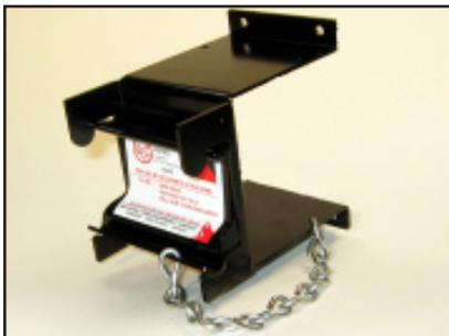
**Application:** Used with S-4 pin racks to provide one man operation of fire hose. Model S-5 hose water-stop clamp allows valve to be opened without the flow of water until the last fold is removed and hose is pulled from nozzle end. For 1 ½" (38mm) single jacket lined hose only.
