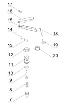
\* NOTE - Valve Body Assemblies include: Top Lever, Carry Handle, 3 x Rivets, Valve Body (w/ Schrader Valve), Gauge, Valve Body Collar, O-Ring, Pull Pin & Retaining Strap
