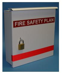
Our Fire Safety Plan box is made 18 gauge Satin Coat Steel construction with stainless steel rivets and piano hinge, weather proof door seal, overhanging sill and UV resistant decal for maximum weather protection and durability.
